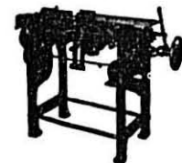
PETERS JUNIOR CARTON FORMING AND LINING MACHINE (above) sets up 35-40 cartons per min., one operator.
